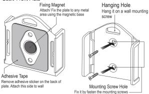
• Bracket + XHLogger Place the XHLogger into the mounting bracke
