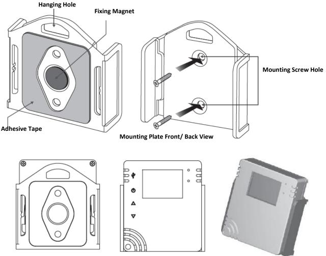
Mounting Plate Front/ Rear View with XH Installed
